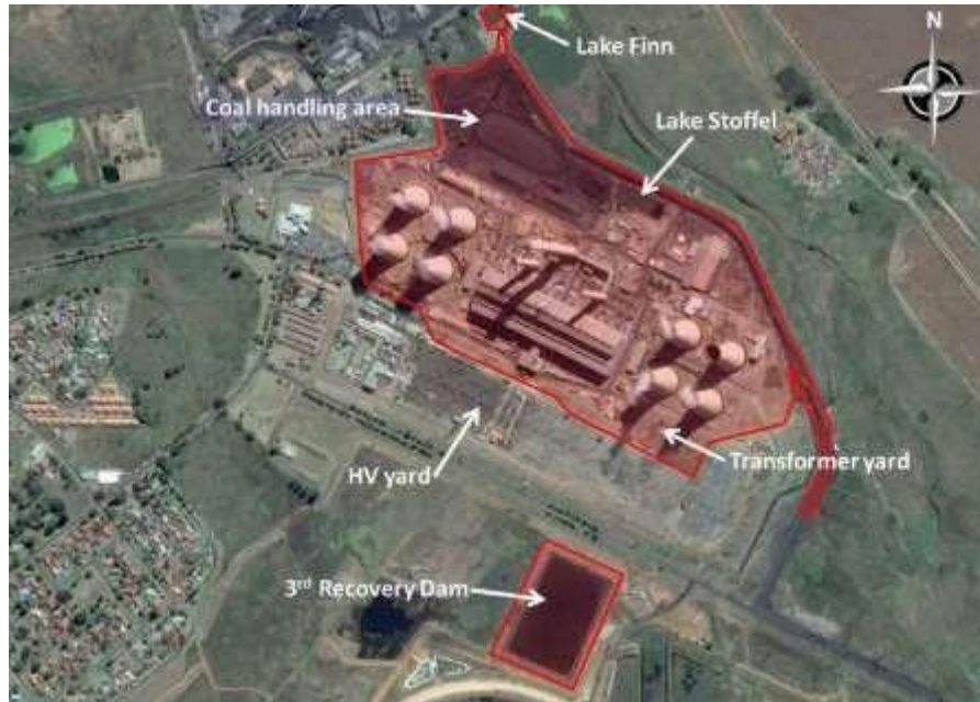
Figure 3: Pollution Control/Effluent Collection dams and catchment areas
